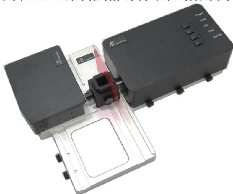
Figure 4-2: Absorbance/Transmittance measurement example thin film
