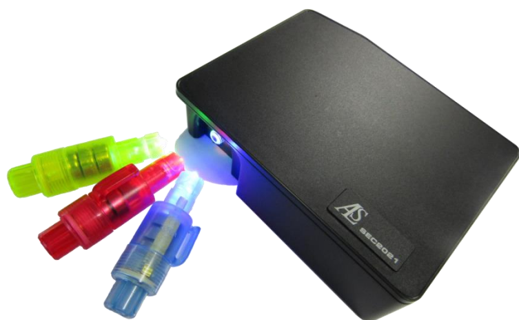
Figure 7-1: Emission intensity measurement of LED lamp
