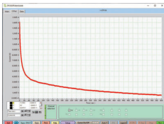
Fig. 3-1. Constant potential electrolysis for 2 mM potassium ferrocyanide.
