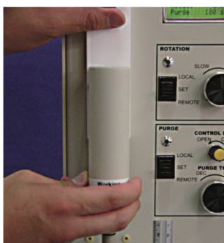
Figure 5-6-1 Fasten the knob of RRDE-3A, and Teflon plate moves up.
