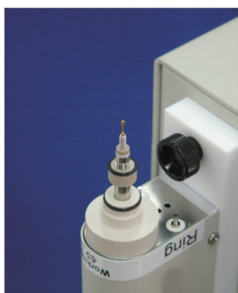
Figure 5-6-4 Now the contact pin is positioned at the top. Pin is sharp, handle with care. RDE or RRDE is mounted here.
