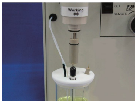
Fig 3-8-4. Six holes are located on the Teflon cap. These holes are for the reference, counter, working electrode and purge tubes. Place the electrodes in the most convenient way. The last hole is for the gas outlet.
