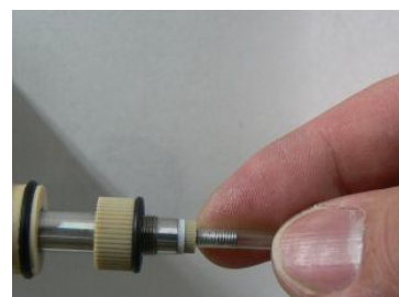
6-8-3. Put a new Heat shrink tubing on the tip of the shaft assembly .
