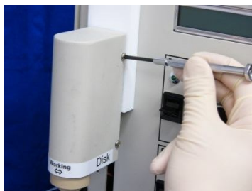
6-5-1. Unscrew four metal screws, which are used for fastening the white motor assembly cover of RRDE-3A, with a screwdriver (#1 or #2).
