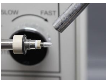
6-8-4. Shrink the tubing to wrap the shaft with heat gun or a drier (by 150 degrees Celsius)
