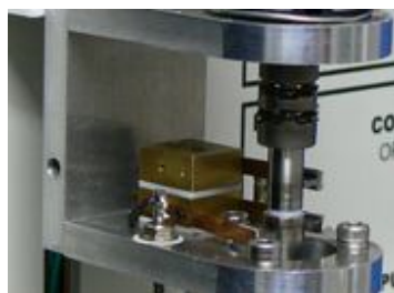
6-5-4. Remove the old silver-carbon brush unit and put the new one on the brush base.
