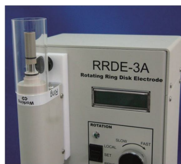
Figure 5-6-6 It's ready for spin coating experiment. A sample you want to coat is dropped on RDE or RRDE. The motor is rotated for a few minutes, then the chemically modified electrode with a constant membrane thickness is available.
