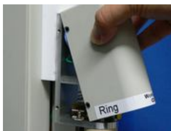
6-5-2. Remove the motor assembly cover.
