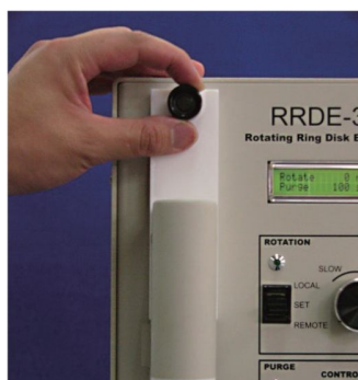
Figure 5-6-2. Fixe the Teflon plate at the top position.
