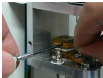
6-5-5. Make sure to fix the new silver-carbon brush unit with tiny screws.
