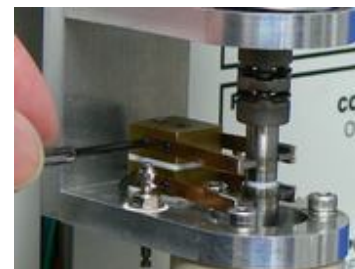
6-5-3. Unscrew two tiny screws connecting between the brush base and the bad silver-carbon brush unit with a screwdriver (#000).
