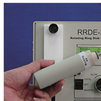
Figure 5-6-3 Rotate at 180 degree the motor housing
