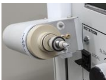
6-7-5. Stick the new probe into the hole of the shaft .
