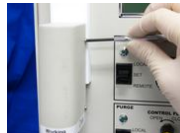
6-5-6. Put the motor assembly cover and fix it.
