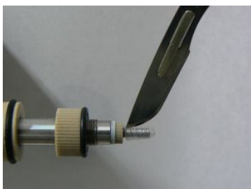
6-8-1. After taking out the probe cut the Heat shrink tubing with a knife.
