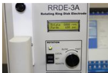
6-5-7. Please rotate the rotator by 8000 rpm for 10 minutes for making the low resistance between silver-carbon brushes and shaft and for turning down the noisy sound during rotation.
