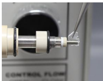
6-8-2. Remove the Heat shrink Teflon tubing like peeling.
