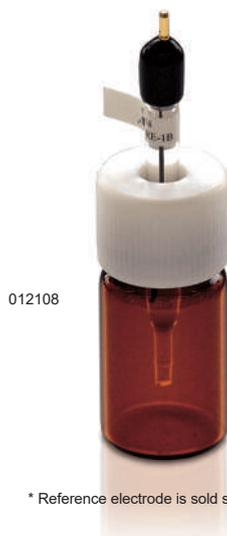
If purchased or self-prepared reference electrode is left in direct contact with air, the inside solution will evaporate and dry up gradually. When it is not in use, a recommended way, in order to maintain the reference electrode capability and life time, is to preserve in a sealed preservative bottle with a solution, similar to the reference electrode internal solution.
