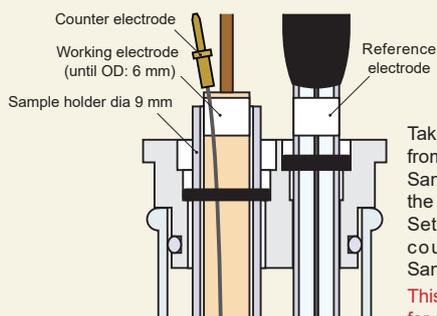
Take out the Teflon cap adaptor from the Teflon cap, and set the Sample holder of the 9.0 mm of the diameter (optional item). Set the working electrode and counter electrode into the Sample holder.
