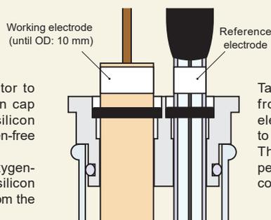
Take out the Teflon cap adaptor from the Teflon cap. Working electrode can be fitted directly to the Teflon cap. The O-ring will fit perfectly. It permits to have the oxygen-free condition.
