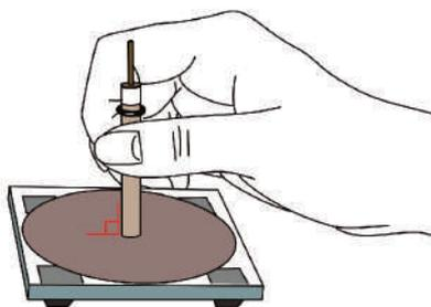
Hold the CV electrode at right angle to the pad.
