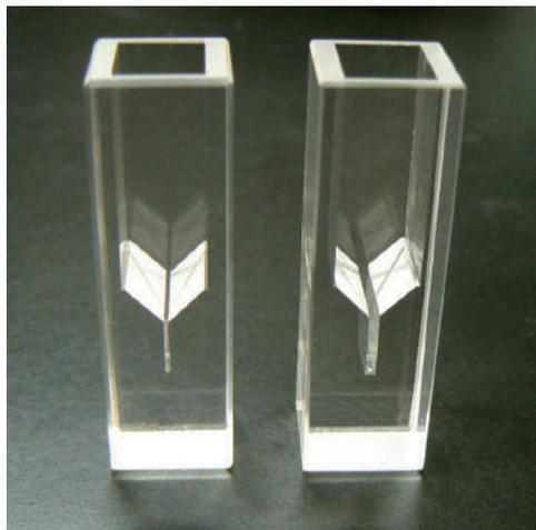
The electrolysis time for the 0.5 mm optical path length cell is theoretically a half, compared with the 1.0 mm cell. It is the opposite, for the concentration, when the same result for the 1.0 mm cell is possible for a half of the concentration compared with the 0.5 mm cell. You could select the optical path length and the working electrode appropriate for your research purpose.
