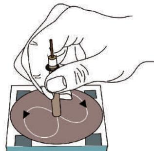
Polish in a circular motion, for 30 seconds to 2 minutes. Rinse the electrode surface with distilled water.
