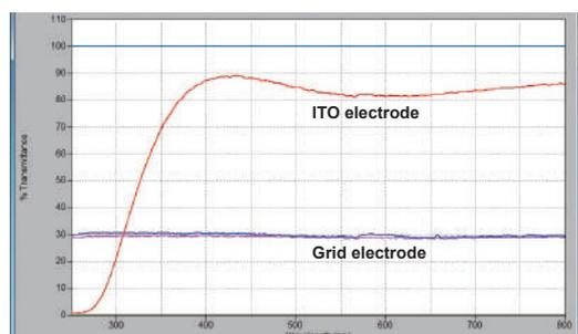
The light transmittance was compared with ITO electrode and Grid electrode (Au, Pt and Carbon) on a quartz glass as a reference. For ITO electrode the light cannot be transmitted easily in an ultraviolet range. The transmittance is about 10% at 280 nm of the wavelength. For wavelength above 400 nm the transmittance is above 80%. Compared with the quartz glass, the light transmission for grid electrode is about 30%, however it could be used in an ultraviolet range.
