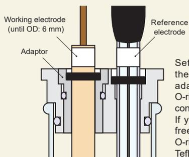
Set the Teflon cap adaptor to the Teflon cap. The Teflon cap adaptor is fixed with a silicon O-ring to work in an oxygen-free condition. If you do not need the oxygen-free condition, then the silicon O-ring can be taken out from the Teflon cap.
