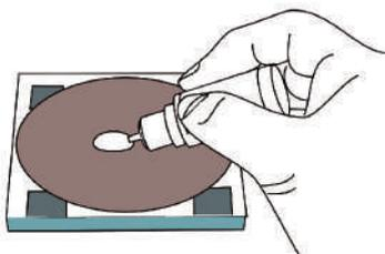
Prepare the glass plate, and put a few drops of polishing diamond on diamond polishing pad.
