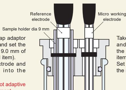
Take out the Teflon cap adaptor, and set the Sample holder of the 9.0 mm diameter (optional item). Set the reference electrode into the sample holder.
