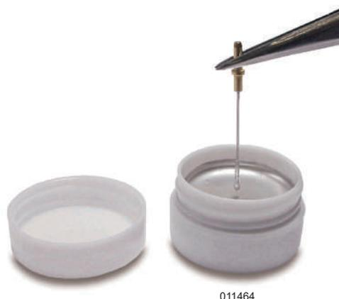
Reference electrodes can be easily prepared by coating Ag/AgCl ink on the metal (Ag, Pt, Au, etc.) surface. The only thing you are required to do is just to deposit the Ag/AgCl ink and wait for dry. The reference electrode prepared by Ag/AgCl ink is quite useful for IDA electrode measurements.
