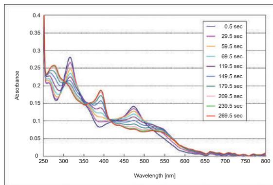
Fig.4-2. Electrolysis spectrum change of Vitamin B<sub>12</sub> derivative complex.
