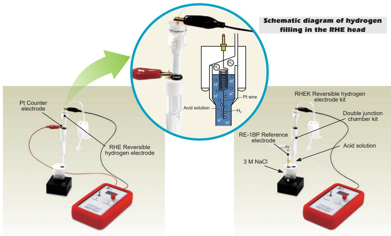
**Schematic diagram of hydrogen filling in the RHE head**
