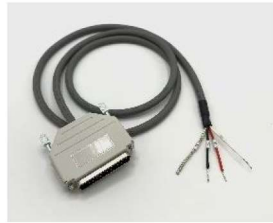
Figure 1-1 CB-ES Remote cable(25pin)
