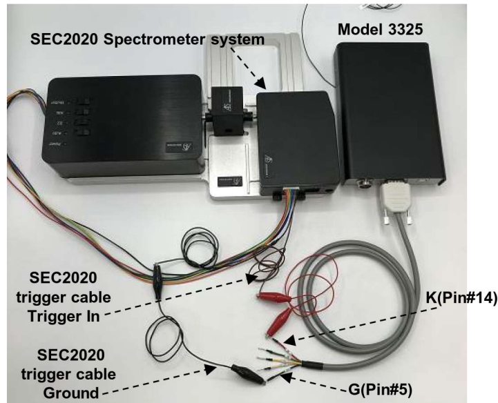
Figure 3-1 Trigger connection of Model 3325 and SEC2020
