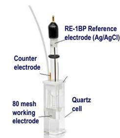
4. SEC-CT Thin Layer Quartz Glass Spectroelectrochemical cell kit (Pt)
