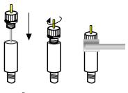
1-2. Insert the cap into the sample holder, and fasten the cap tightly. Seal the cap to avoid evaporating of the inner solution.
