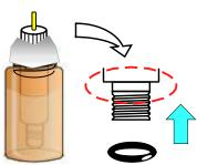
1-3. Soak the reference electrode in electrolyte solution for 1 day. After soaking, wipe out the adherent solution and set the O ring on the tip of sample holder.
