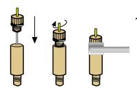
1-2. Insert the cap into the sample holder, and fasten the cap tightly. Seal the cap to avoid evaporating of the inner solution.
