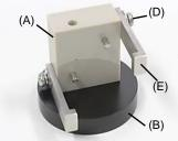
1. A cross flow cell block(A) is attached to a flow cell base block(B) with screws(C) from the bottom of the flow cell base block (B), and flow cell arms(E) are connected to the cross flow cell block(A) with screws(D). Please use a Phillips screwdriver for assembly.
