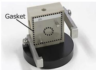
2. A gasket(option) is put on the electrode block as shown the figure to the left.
