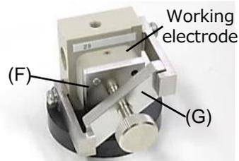
3. The electrode surface of a working electrode(option) is put on the hole of the gasket,, and the stainless plate for clamp(F) is put and fixed as the left figure in the clamp(G).
