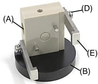
1. The radial flow cell block(A) is attached to the flow cell base block(B) with screws(C) from the bottom of the base, and flow cell arms(E) are connected to the electrode block with screws(D). Please use the Phillips head screwdriver for the assembly.
