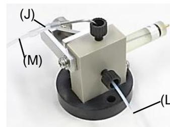
5. The Teflon tube(L) is connected with a fitting. Put the silicone tube(J) on the tip of the stainless pipe and connect the Teflon tube (M).
