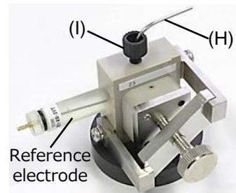
4. A reference electrode(option), a fitting PEEK(I), and the stainless pipe 5cm(H) are attached as the left.
