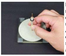
Press the electrode to the pad at right angle, and polish in motion of drawing 8 shape for few minutes under vertical state.
