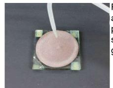
Replace the diamond pad with an alumina polishing pad, wet the pad with distilled water, remove surplus water by fingers (clean glove wearing).
