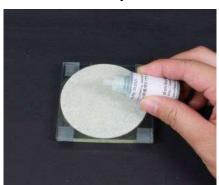
Paste the diamond polishing pad onto the glass plate. Then drip 2~3 drops of polishing diamond to the pad and add 2-3 drops of distilled water before polishing.
