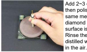
Add 2~3 drips of polishing alumina, then polish the electrode by the same method to that using diamond polishing, until the mirror surface is regenerated.
