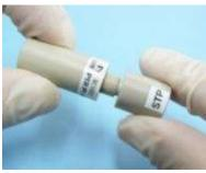
2-2. Push the silicone rod into the ring assembly by using DRE-STP slowly. Be care to keep the silicone rod surface at the flat or slight lower position of the Pt ring surface.
