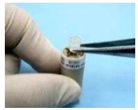
2-1. Cut the silicone rod into 0.5 cm and insert into assembly with the contact side.
