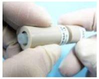
2-3. After polishing, screw in the DRE-STP to push out the silicone rod and remove it from the electrode side. DRE-STP must be used for removing the silicone rod. Any Pt ring damage due to use of other tool to remove the silicone rod is out of guaranty range.
