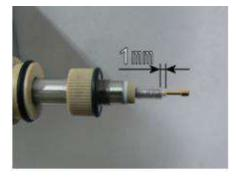
2-5. Cut the contraction tube at the position 1 mm longer than the shaft tip. Insert the contact probe into the shaft contraction tube fully.
