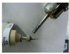
2-4. Thermal shrink the contraction tube with heat gun or dryer (temperature higher than 150 °C).
