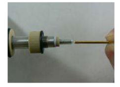
1-1. The first step is drawing out the contact probe from the shaft contraction tube.
