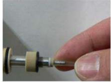
2-3. Cover the shaft tip with a new contraction tube. (Advice: If the tube was tight for shaft tip, Please turn the tube in the direction of the shaft tip screw threads.)
