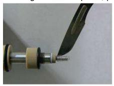
2-1. Remove out the contact probe firstly, then cut the shaft contraction tube carefully.
