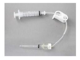
Connect the accessories kit to RHE reversible hydrogen electrode like left figure.
