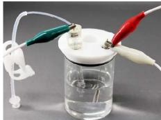
Connect the working electrode cable to RHE, and connect the reference and counter electrode cable to the Pt counter electrode. Electrolyze the acidic solution until 2 coulomb electric charges pass. (For example: apply -3V vs. ref to WE for about 5 minutes in 1.2 M HCI solution.)
