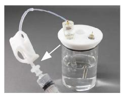
Leave the tubing clamp at open state. Use the disposable syringe and suction the acidic solution gently till the solution is near the female lure fitting and close the tubing clamp firmly.
