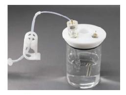
Prepare a Pt counter electrode (options: 012961, 002222 etc.) and set it together with a RHE to the electrolysis cell which filled with acidic solution.
