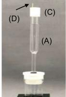
2-2. Attach a PTFE Cap(C) to the double junction chamber (A), set the Platinum counter electrode 5.7 cm(D) to the PTFE Cap(C)
