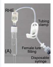
2-3. Set RHEK Reversible hydrogen electrode kit (sold separately) to the double junction chamber(A). With a tubing clamp open, use a disposable syringe to suck the acidic solution from RHE until it reaches the disposable syringe. Make sure that there are no air bubbles between the female lure fitting and then tighten the tubing clamp.
