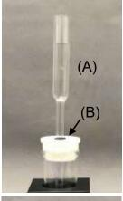
2-1. Set an O-ring(B) on a double junction chamber(A). Stand the double junction chamber(A) and inject the acidic solution gently along inside wall. The suitable liquid volume for the double junction chamber(A) is 4.5 mL.
