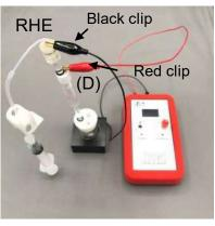
2-4. Prepare an H2G1 Portable Hydrogen Generator and connect a black clip to the RHE and a red clip to the Pt counter electrode(D). Filling time is approximately 4 minutes with 1.2 M HCl. For using a potentiostat, please refer to following website for details. https://www.als-japan.com/RHE.html.
