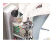
5. Turn over the motor unit and wipe the dirt from the contact surface of the frame plate and bearing assembly.
