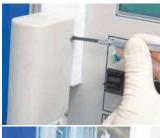
Move the motor unit to top position, remove 4 screws on the motor cover with Philips screwdriver (#1), then take off the cover from the motor unit.
