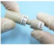
Step-2. Push the silicone rod into the ring assembly by using DRE-STP slowly. Be care to keep the silicone rod surface at the flat or slight lower position of the GC ring surface.(DRE-STP is a content of 013608 DRE-DCP)
