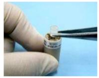
Step-1. Cut the silicone rod into 0.5 cm and insert into assembly with the contact side.
