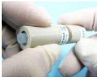
Step-3. After polishing, screw in the DRE-STP to push out the silicone rod and remove it from the electrode side.
