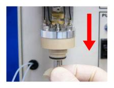
3.Pull out the shaft gently. If the shaft gets stuck with the carbon brush, loosen the brush fixing screws or expand the brush head by tweezers. (NOTE: If the shaft is severely damaged and cannot be pull out easily, please remove the bearing assembly in advance, then remove the shaft together with the bearing.)
