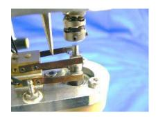
4.Insert the new shaft gently through the bearing while loosening carbon brush screws or pulling the carbon brush with tweezers.
