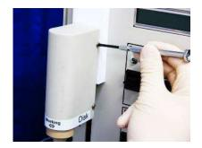
1.Remove the screws by using the Phillips screwdriver(#1) for detaching the cover of motor unit.
