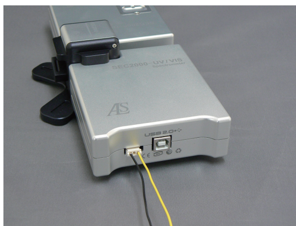
Fig. 2 The external trigger cable. The black wire is for Ground, and the yellow wire is for Trigger In.
