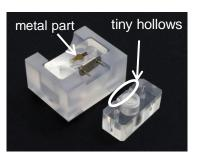
Put the Metal part of the quartz crystal oscillator (optional) to the center of the Oring (I) on the EQCM flow cell (A). Put on the EQCM cell (B) carefully with making its tiny hollows face same direction. Check the terminal pin connecting with the metal part that touch the sample solution.
