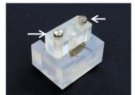
3. Fix two cells (A&B) with two fixing screws (J). Gradually tight two screws in turn with nice balance.
