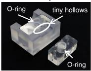
Put the EQCM flow cell (A) into the cell holder (C) by facing the side of two tiny hollows (in half cylinder shape) of A to the side of small dent (in shallow step shape) of C. Set the silicon O-rings (I) into the center hole of EQCM flow cell (A) and EQCM cell (B) respectively.
