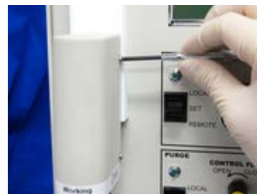
Fig. 6-5-6 Put the motor assembly cover and fix it.
