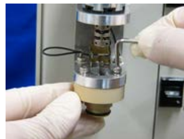
Fig. 6-9-6 Rotate the housing back to initial position and attach the new bearing assembly with hex key carefully.
