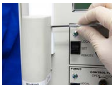
Fig. 6-6-8 Enclose the shaft with white cover and then, fix it by four metal screws, with a screwdriver (#1 or #2).
