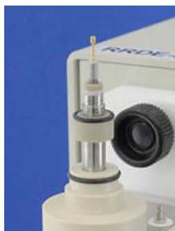
Fig. 5-6-4 Now the contact pin is positioned at the top. Pin is sharp, handle with care. RDE or RRDE is mounted here.
