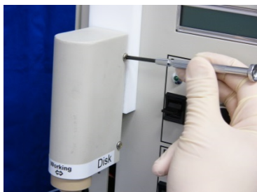
Fig. 6-9-1 Unscrew four metal screws, which are used for fastening the white motor assembly cover of RRDE-3A, with a screwdriver (#1 or #2).
