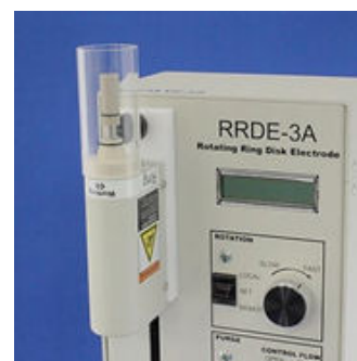
Fig. 5-6-6 It's ready for spin coating experiment. A sample you want to coat is dropped on RDE or RRDE. The motor is rotated for a few minutes, then the chemically modified electrode with a constant membrane thickness is available.
