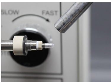
Fig. 6-8-4 Shrink the tubing to wrap the shaft with heat gun or a drier (by 150 degrees Celsius)
