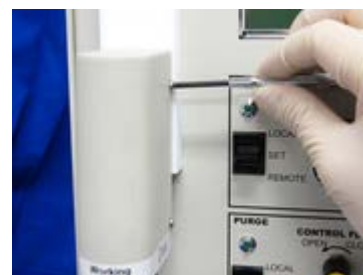
Fig. 6-9-9 Enclose the shaft with white cover and then, fix it by four metal screws, with a screwdriver (#1 or #2).
