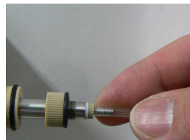
Fig. 6-8-3 Put a new contraction tube on the tip of the shaft assembly.
