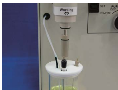
Fig. 3-8-4 Six holes are located on the Teflon cap. These holes are for the reference, counter, working electrode and purge tubes. Place the electrodes in the most convenient way. The last hole is for the gas outlet.
