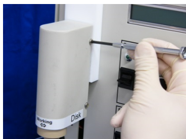
Fig. 6-6-1 Unscrew four metal screws, which are used for fastening the white motor assembly cover of RRDE-3A, with a screwdriver (#1 or #2).
