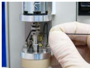
Fig. 6-9-8 Screw two set screws on the lower side of the flexible coupling with hex key (0.89 mm = 0.035 inch).
