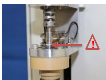
Fig. 6-6-6 Please bend the silver-carbon brushes for ring electrodes toward the outside slightly with tweezers again, to let pass the gap between Teflon separator and lower side of the shaft .
