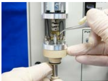
Fig. 6-9-7 Stick the new shaft into the hole of the bearing and lift it up carefully while bending the leaf spring of silver-carbon brush toward the outside slightly with tweezers.
