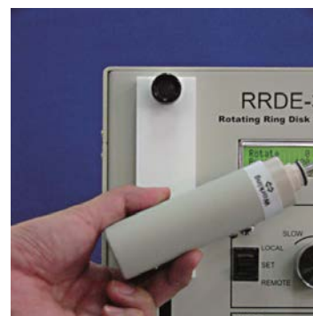
Fig. 5-6-3 Rotate at 180 degree the motor housing
