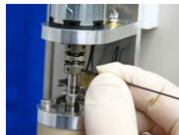
Fig. 6-6-3 Loosen the second screw on the lower side of the flexible coupling until the shaft is released, while holding the shaft with another hand.
