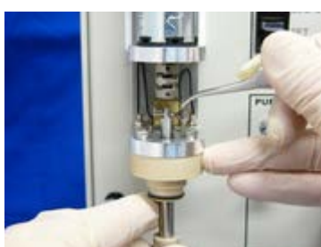
Fig. 6-6-5 Stick the new shaft into the hole of the bearing and lift it up carefully while bending the leaf spring of silver-carbon brush toward the outside slightly with tweezers.
