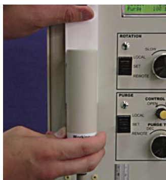
Fig. 5-6-1 Fasten the knob of RRDE-3A, and Teflon plate moves up.
