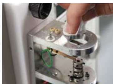
Fig. 6-9-5 Rotate the motor housing at 180 degree and wipe the bottom of the aluminum frame with some swab or paper.
