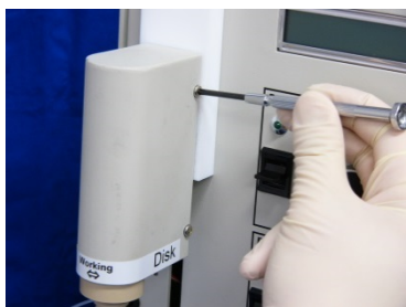
Fig. 6-5-1 Unscrew four metal screws, which are used for fastening the white motor assembly cover of RRDE-3A, with a screwdriver (#1 or #2).
