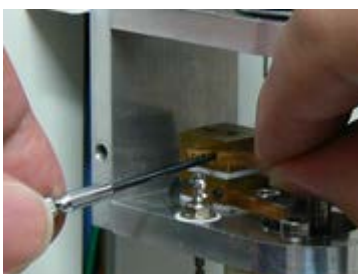
Fig. 6-5-5 Make sure to fix the new silver-carbon brush unit with tiny screws.
