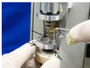
Fig. 6-9-4 Remove the bearing assembly by loosening three set screws connecting between the aluminum frame and the bearing with hex key (2.5 cm).
