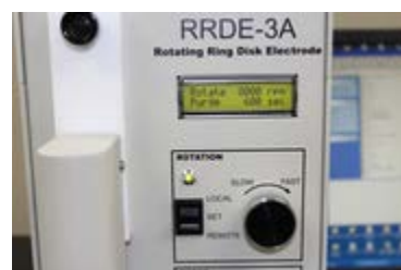
Fig. 6-5-7 Please rotate the rotator by 8000 rpm for 10 minutes for making the low resistance between silver-carbon brushes and shaft and for turning down the noisy sound during rotation.
