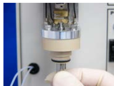
Fig. 6-9-3 Pull the shaft gently. If the shaft does not go out smoothly because of silver-carbon brushes , please release them by loosen the tiny screws, or bend the leaf spring for silver-carbon brush with tweezers, slightly.
