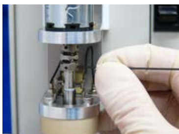
Fig. 6-6-7 Screw two set screws on the lower side of the flexible coupling with hex key (0.89mm = 0.035inch).
