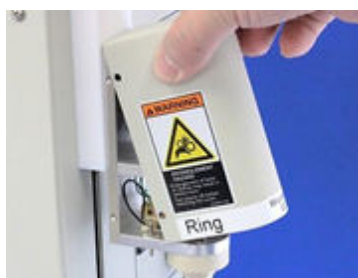
Fig. 6-5-2 Remove the motor assembly cover.
