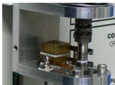
Fig. 6-5-4 Remove the old silver-carbon brush unit and put the new one on the brush
