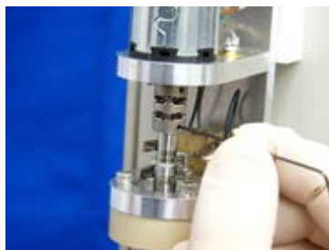
Fig. 6-9-2 Loosen screw pair on the lower side of the flexible coupling with hex key (0.89 mm = 0.035 inch) until the shaft is released, while holding the shaft with another hand.
