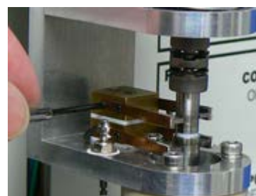
Fig. 6-5-3 Unscrew two tiny screws connecting between the brush base and the bad silver-carbon brush unit with a screwdriver (#000).
