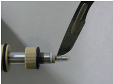
Fig. 6-8-1 After taking out the probe cut the contraction tube with a knife.
