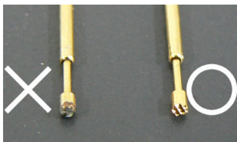
Fig. 6-7-1 Corroded probe on the left
