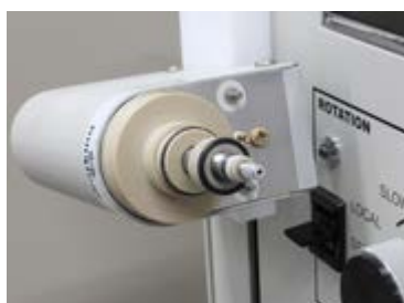
Fig. 6-7-5 Stick the new probe into the hole of the shaft .
