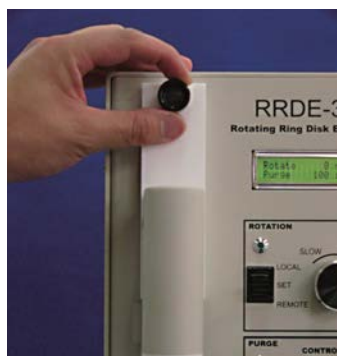
Fig. 5-6-2. Fixe the Teflon plate at the top position.
