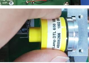
Plug the power terminals of halogen bulb.
