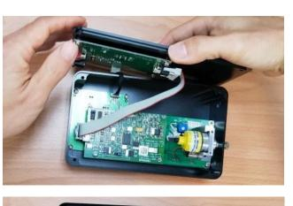
Disassemble the bottom cover. (It is no need to disassemble the cable)
