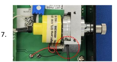
Unscrew the hexagon socket set screw (marked by  $\bigcirc$ ) by using hex wrench.
