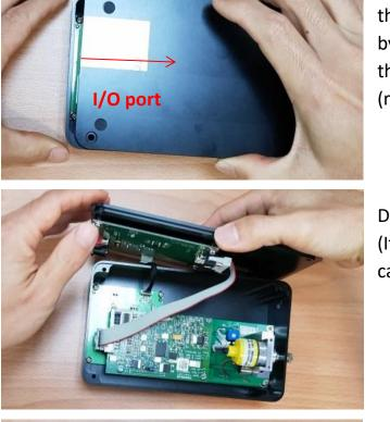
Because the I/O port is in the hole on the side of the chassis, open the cover by slightly shifting the bottom cover in the direction opposite to the I/O port (right direction in the picture).
