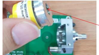
Remove the bulb and install a new replacement bulb.
